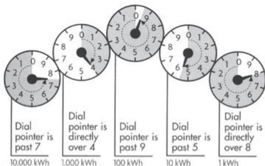
As an example, the reading from the dial pictured is 74958. If a nine follows any number underlined, (i.e. the 4) reduce that figure by one. The correct reading on this meter is 73958.
